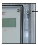
Screw in through holes provided outside of the rubber seal.
