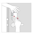
Once confirmed with the appropriate height of the stand, screw all the screws and close the battery case cover.
