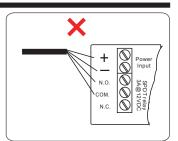
Do not run power wires and signal wire in the same cable or conduit.
