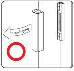
**Note:** For security reason, it is recommended to install the PH series on the in-swinging doors instead of out-swinging doors from potential damage due to intruders or vandals.
