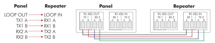
If there is more than 1 repeater, continue to connect OUT of one Repeater to IN of the next Repeater following the same connection rules as above. When you reach the last Repeater in the loop make the connections as follows:
