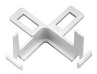
**CB500 Control Module Barrier** Separates power limited wiring from non-power limited wiring in control module applications
