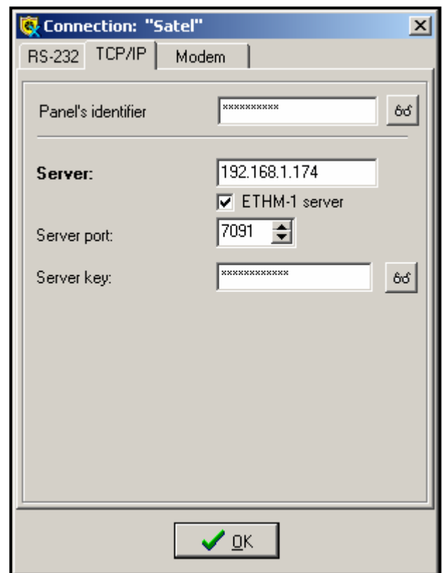
Fig. 6. Window with an example of configuration of TCP/IP connection in GUARDX program.
