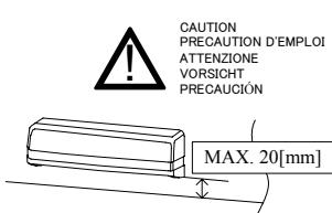
**EN** Mounting higher will render the sensor unable to detect the door rail area.
