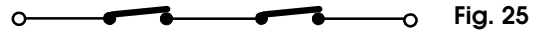
Connection of two N.C. contacts in series (e.g. Photocells, Stop, Edge, etc.)
