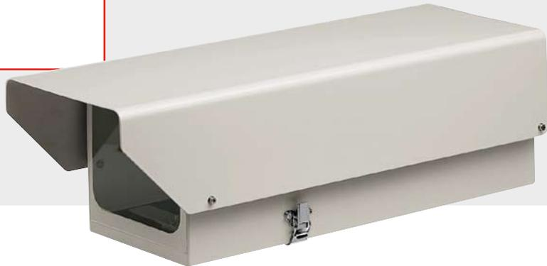
The NXJ housing, entirely made of AISI 304 stainless steel, has been designed to accommodate large cameras and zoom lenses. The NXJ housing has a frontal section of 180x170mm and is 500mm in length. It consists of a base with internal slide and a body which closes by means of three fastening clips.
