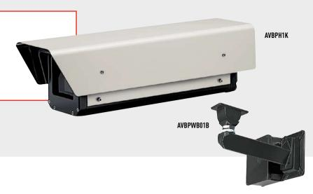
Armoured housing, consisting of a 10mm thick extruded aluminium base with front and rear bottom made of 30mm thick die-cast aluminium. An 18mm-bullet-proof glass is fixed on the front by means of an iron frame. The armour plating is made of 3mm stainless sheet steel, which covers the base and housing body.
