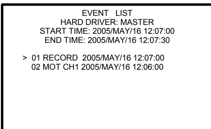
Use the ▲ and ▼ keys to scroll the cursor until it reaches the desired event. Press “PLAY” to show the corresponding recording.
