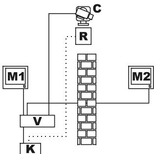
In this example keyboard K directly controls receiver R to move camera C.
