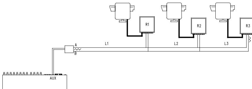
Receivers R1, R2 should not have the termination resistance inserted. The maximum length of the line, from end to end (from the matrix AUX line to receiver R3), is 1200 metres.
