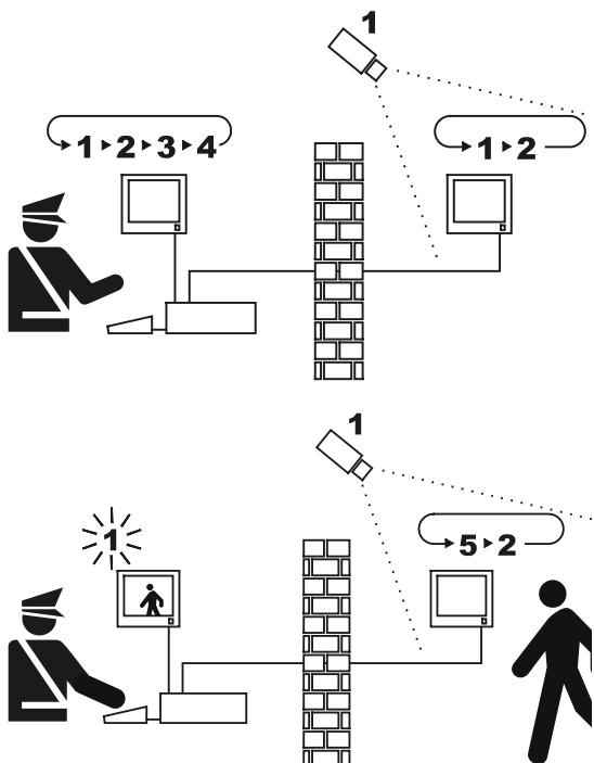
In the example the master monitor shows a switching sequence on inputs 1, 2, 3 and 4. The public monitor shows inputs 1 and 2. Camera 1 frames the area including the public monitor.
