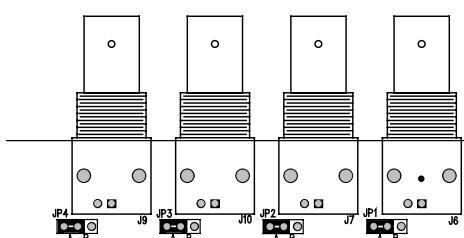
Example: all input with 75 Ohm load inserted
