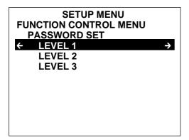
**3** Highlight the level for which a password is to be set, then press the → key.
