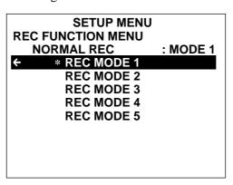
4 Highlight the desired recording mode, REC MODE 1 to 5 (or display Mode 1 to 5) by pressing the ★ or ★ key, then press the SET key.
