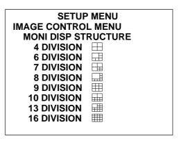
**3** Highlight the desired division mode by pressing the ♠ or ♦ key, then press the ▶ key.
