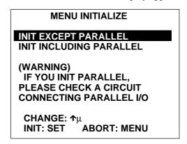
2 Specify whether to initialize the menu except the parallel input/output settings or to initialize the menu including the parallel input/output settings.
