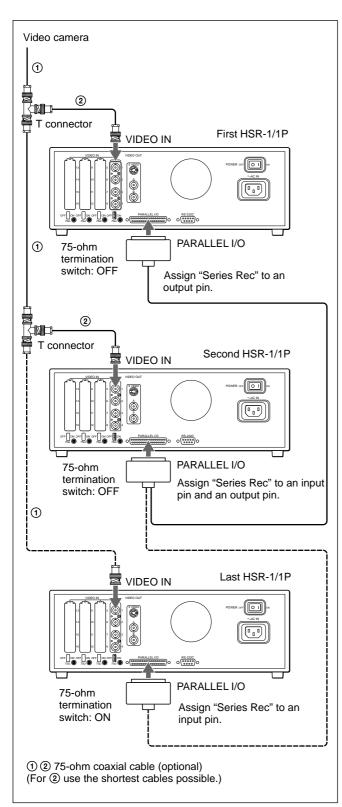
For pin assignment of the PARALLEL I/O connector, see "Remote Control Menu" on page 4-13.
