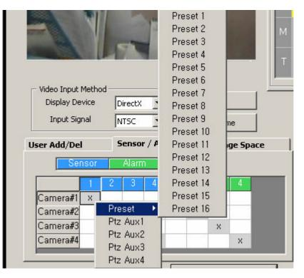
"P1 ~ P16": When sensor works, camera operates to preset location.
