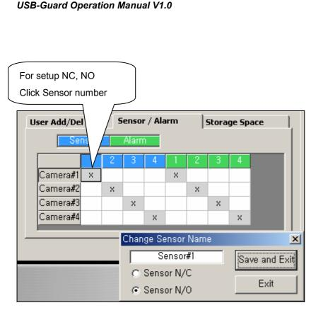
You can set NC (Normal Close), NO (Normal Open) and Alarm out duration. Digital out is worked by event on schedule, during how long time you set. It's not worked when you switched digital out.
