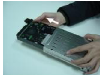
Step 5 Remove the HDD from Cartridge
