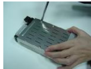
Step 4 Loose all screws on the Cartridge
