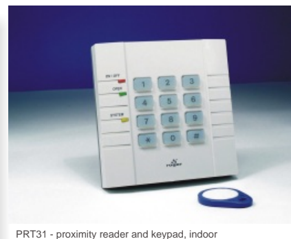
PRT31 - proximity reader and keypad, indoor
