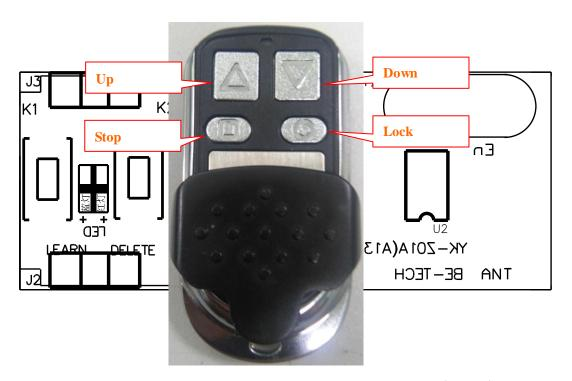
Our factory design and produce the tube motor controller (YET863), this kind of wireless receiving control is high stable characteristics, low power consume and very convenience, it is unnecessary adopt the traditional wire jumper or dip switch code but only receive and store the wireless signal from the remote control, and it can match with remote control.
