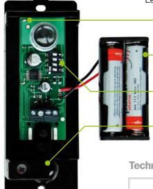
Led indicator to simplify the alignment of the photocells
