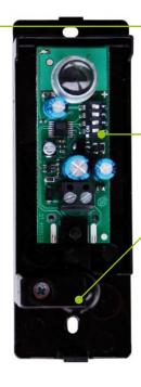
LED indicator to simplify the alignment of the photocells
