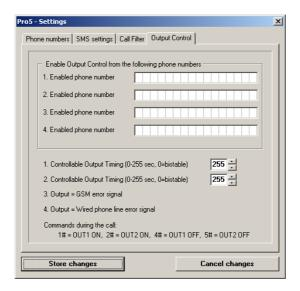
Remote control will be reachable from the numbers set here. If there is an incoming call from any of the here given numbers, the module does not forward the call to the security panel or the telephone set, but automatically receives the call. A beep signals ready to use condition in the telephone, and the two outputs can be controlled through the phone by pushing the below mentioned buttons.
