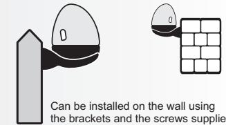
Can be installed on the wall using the brackets and the screws supplied.
