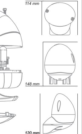
The supplied bracket of the flashing lamp **ONE UP** can host inside the **radio module** cod. RADCN4T (if available). This operation can significantly increase the signal range.
