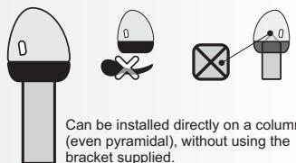
Can be installed directly on a column (even pyramidal), without using the bracket supplied.
