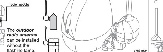
The **outdoor radio antenna** can be installed without the flashing lamp.
