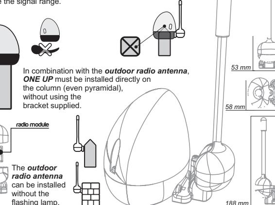
In combination with the **outdoor radio antenna**, **ONE UP** must be installed directly on the column (even pyramidal), without using the bracket supplied.
