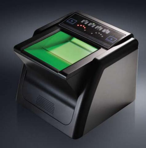
RealScan-10 RealScan-10 is a compact live-scanner for single and ten-print capture. Suprema's advanced optical technology allows high-speed image capturing and seamless image processing. IP54-rated dust and water resistant housing makes it suitable for indoor and mobile environments With its proven reliability of FBI certification, RealScan-10 is the perfect portable live- scanner for civil and criminal applications.
