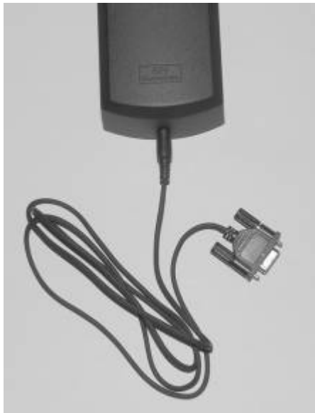
Figure 4> Connecting stereo plug to DB-9 cable
