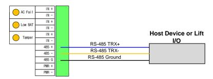
If the communication in the RS-485 is unstable, connect the enclosed 120 Ohm resistor between TRX+ and TRX- connector of Lift I/O for termination.
