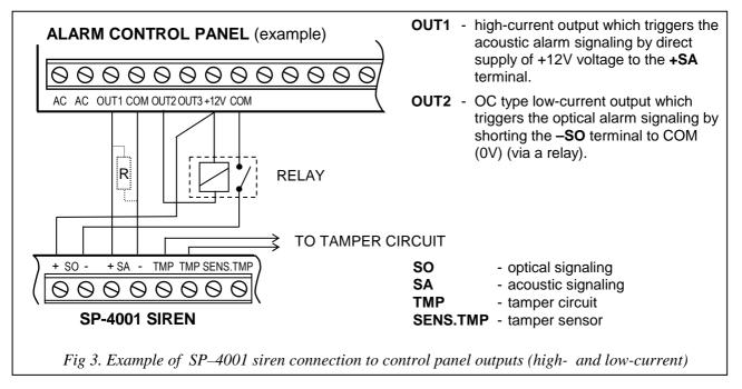
Both types of signaling can be managed from one control panel output if the contacts are connected in parallel i.e. "+SA" with "+SO" and "-SA" with "-SO".
