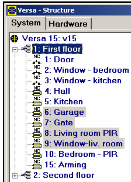
Fig. 6. List of partitions and zones in a tree-like form in the "System" tab, "Versa – Structure" window (an example of configuration).
