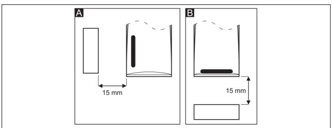
Fig. 3. Max. operation ranges of the reed switches (top view). The indicated ranges are valid for the magnet situated in the presented position, at the height of detector electronics board.
