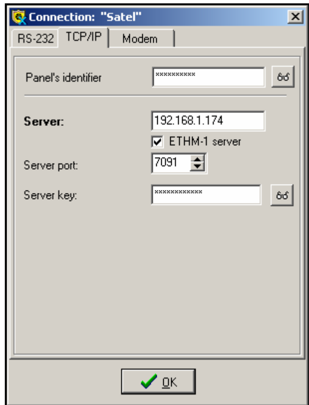
Fig. 7. Window with an example of configuration of TCP/IP connection in GUARDX program.
