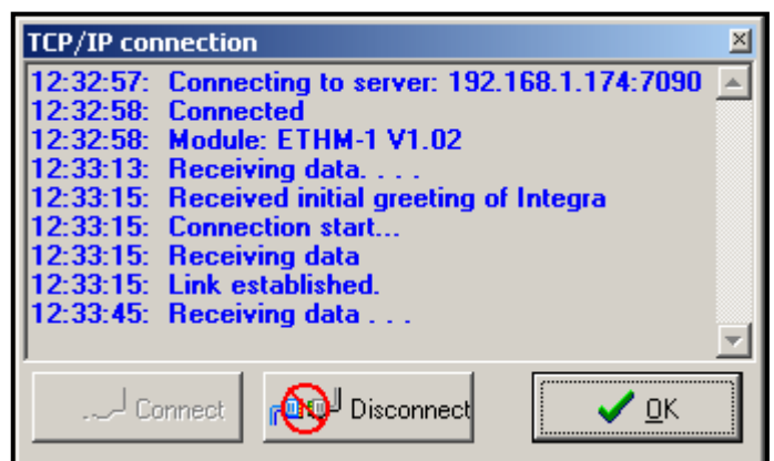
Fig. 6. "TCP/IP connection" window in the DLOADX program, with messages displayed when establishing communication with the panel.
