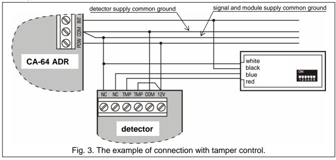
**Note:** Selecting the EOL line type is treated by the control panel as connecting the NC type detector without tamper control.
