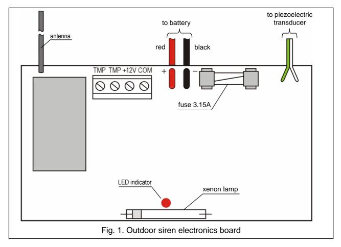
A tamper contact, which reacts to opening or pull-off of the housing from the surface, is connected to the TMP terminals. The terminals +12V and COM are used to connect the outer power supply.
