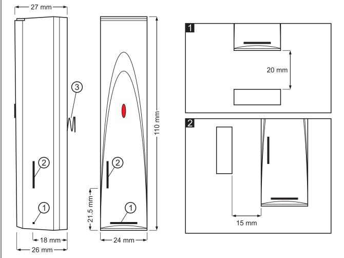
Fig. 2. Housing dimensions, position and maximum operating ranges of reed switches. The shown ranges refer to magnet placed at the height of electronics board.
