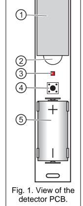
5 - CR123A 3 V lithium battery which ensures operation for approx. 3-year period. The detector controls the battery status. When the voltage drops to 2.6 V, the "low battery" information is sent to the controller. The low battery signaling continues until the battery is replaced.
