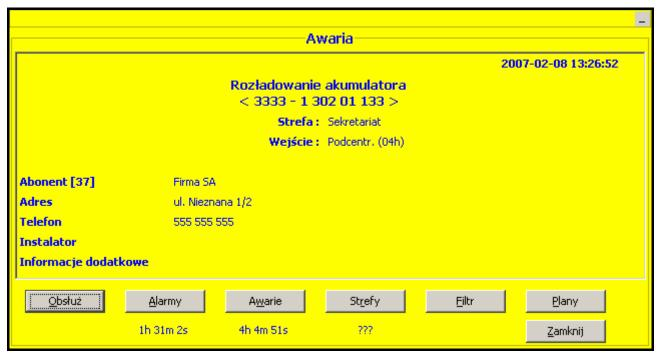
Fig. 35. Example of trouble handling window.
