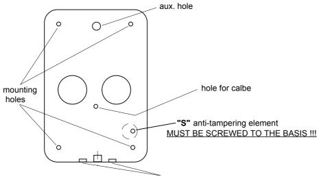
holes for pipeing out the water
