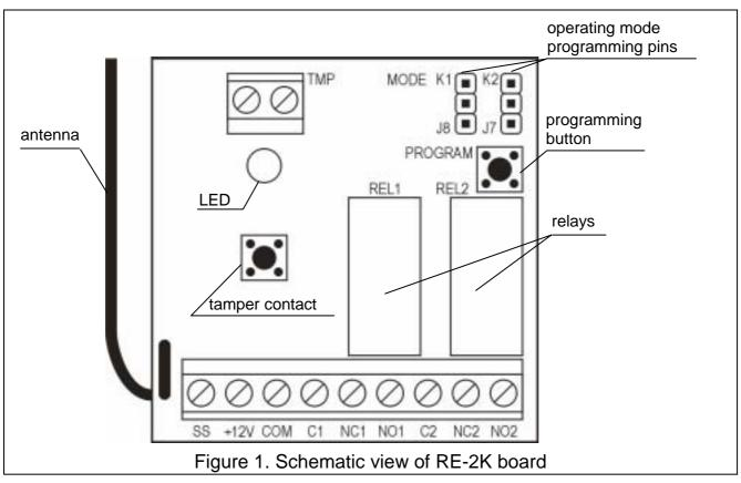
As just one relay is installed on the electronics board of the RE-1 controller, the board has neither the K2 pins or the second relay terminals.
