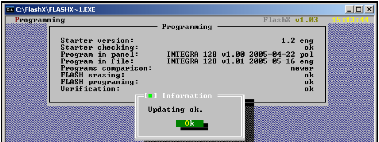
Fig. 9. Message displayed when replacement of the control panel program is complete.
