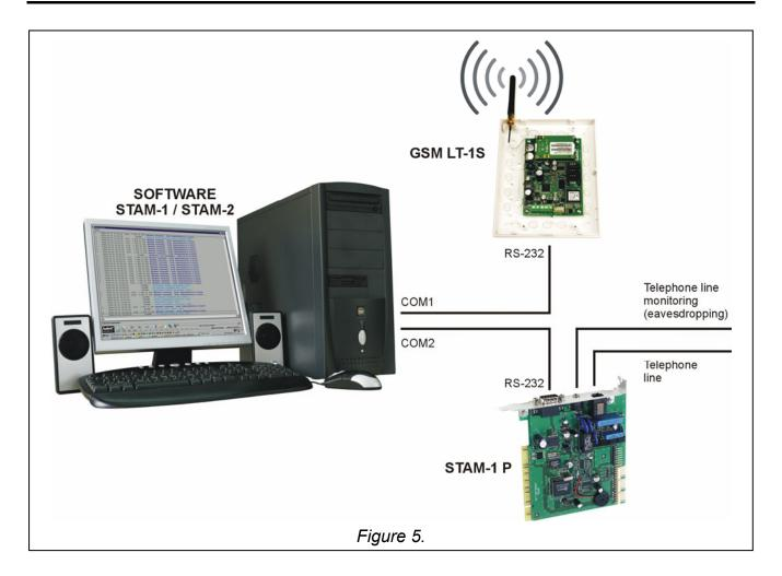
The GSM LT-1S module permits site monitoring by means of SMS short text messages. This function is offered by the STAM-1 monitoring station program, version 4.07 and STAM-2, manufactured by SATEL. The example of module connection to station is shown in Fig. 5. The STAM-1 TRNK expansion board can also be used to connect the module.
