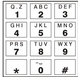
Figure 6. Assignment of alphanumeric characters to telephone keypad.
