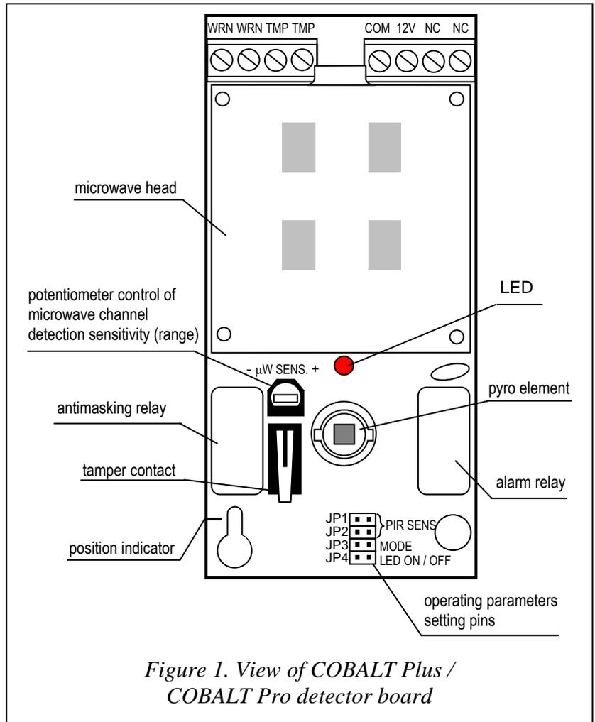
Figure 1. View of COBALT Plus / COBALT Pro detector board
