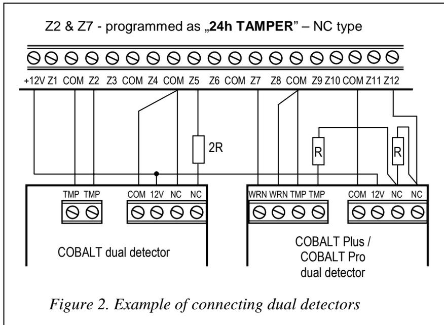
Figure 2 shows typical examples of connecting the detectors in EOL (parameter) configuration and 2EOL (two-parameter) configuration. Resistors should be mounted inside the detector housing.
