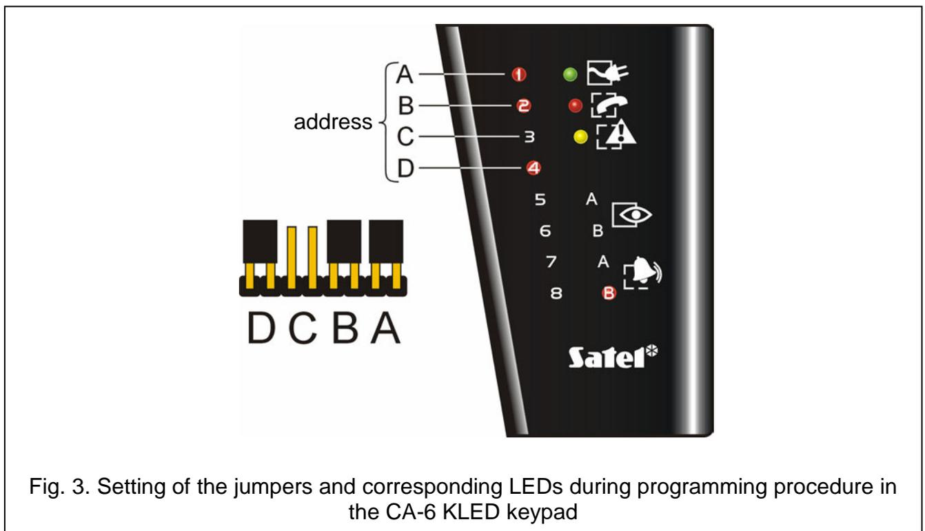
Fig. 3. Setting of the jumpers and corresponding LEDs during programming procedure in the CA-6 KLED keypad
