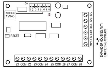
The **set of switches** situated on the board serves to set up the individual expander address. Up to 32 modules of various types can be connected to one bus.
