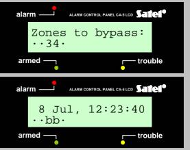
**Note:** The 24h zones (which are on duty, whether the system is armed or not) can only by bypassed by means of the service code.
