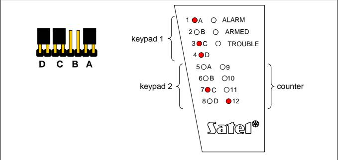
Figure 3. An example of jumper setting in the first partition LED keypad and LED signaling in CA-10 KLED
