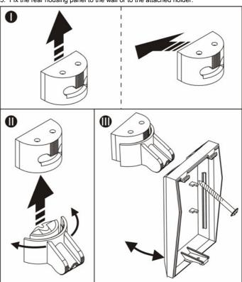
Figure 3. Mounting the detector on the holder.
