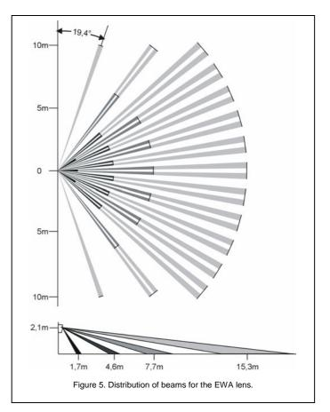
Note: The effective operating range of the detector can differ from the one, which is shown at the figure.
