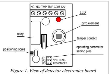
The LED lights red for approx. 2s when the detector is actuated, which enables the installer to check the detector for correct functioning and to approximately determine the protected area.
