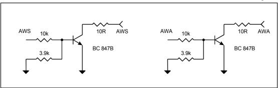
Fig. 2. Diagrams of AWS, AWA outputs
