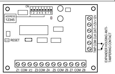
The **set of switches** situated on the board serves to set up the individual expander address. Up to 32 modules of various types can be connected to one bus. Six expander zones can be installed in the system, unless the zones in LCD keypads are used (the total - maximum - number of zones is 64).
