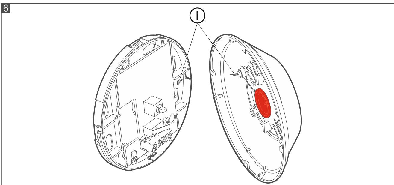
8. Replace the button cover. The marks on the cover and base will help you close the enclosure (Fig. 6).
