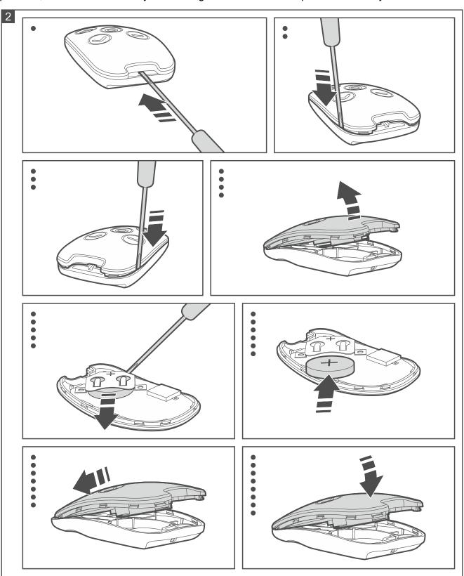
When the battery is low, after pressing the button:
